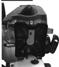
Carefully remove the foam filter insert and check it for damage. Replace if required.
