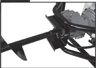
Insert the drive pin. Secure with R-pin.
