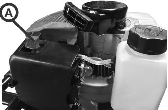
If the engine is cold, move the choke lever (A) to the START position. The choke lever opens and closes the choke in the carburettor.
